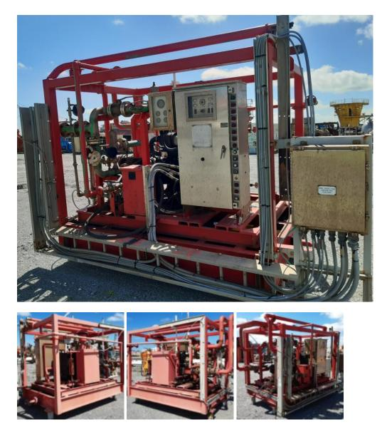
Manufacturer: Edwards-Yanmar Model: 150-338-4TNV88-BDSA Description: Diesel Driven Foam Concentrate Fire Water Pump Package, Running hours 173 Engine, Yanmar Model 4TNV88-BDSA, 35KW Pump, Edwards Model 150-338, 1800Rpm, 150PSI Firetrol Inc. Controller Serial No: 11 2152550-J8935 Condition: Used Stock: 1 External ID: 3267751 Internal ID: 12171 Category: Pumps Subcategory: Pumps, Other Dimension (L x B x H) [m]: 4,10x2,25x2,60 Weight [kg]: 3000
