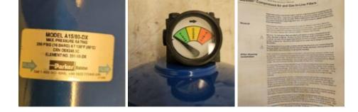
Manufacturer: Parker/Balston Model: D15/80-DX Description: Balston Coalescing Compressed Air Filters protect your equipment and delicate instruments from the dirt, water, and oil usually found in compressed air. Condition: New Stock: 3
